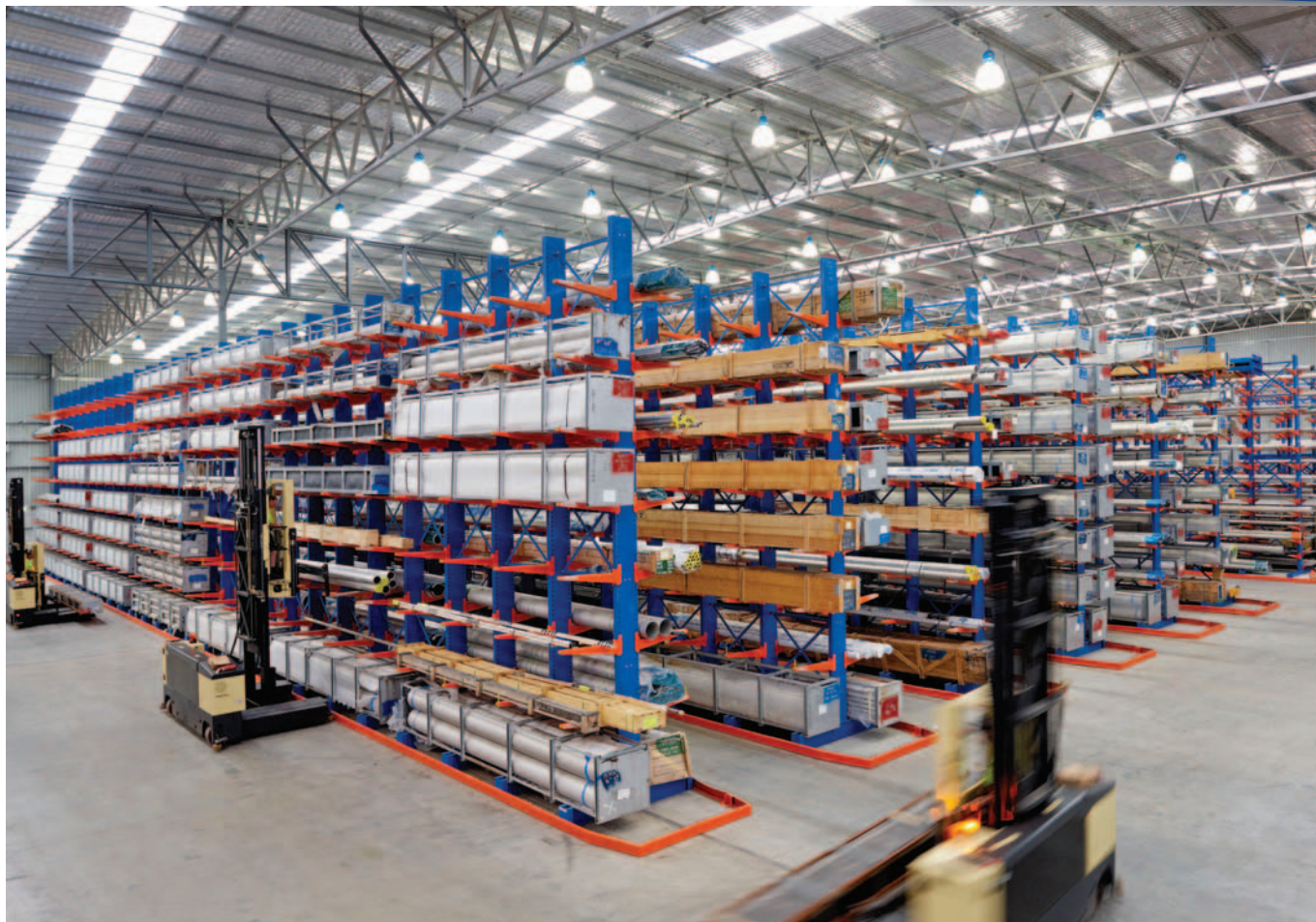
Electronically driven forklift trucks collect pipes, pipe fittings and flanges for delivery to the packaging area.
