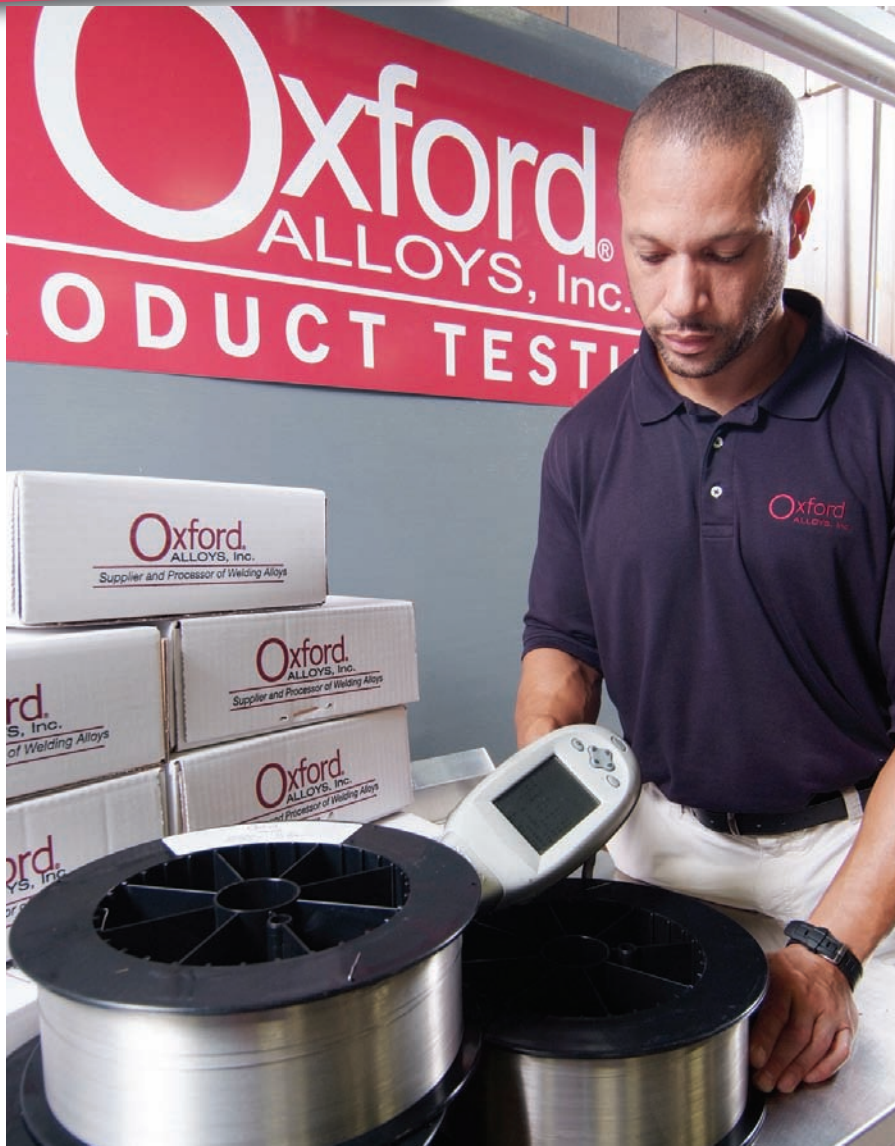
During inspection, top quality testing instruments are used to assure the proper alloy chemistry of each and every heat of material received.
