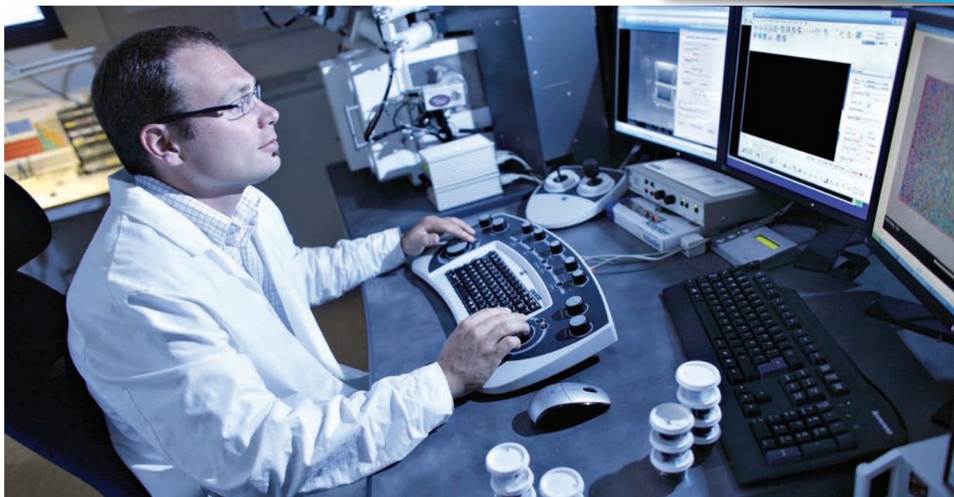
Research Engineer Magnus Boström at the Sandvik R&D center in Sandviken operating a FIB-SEM instrument analyzing the microstructure of high performance stainless steel.
