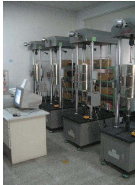
A creep test machine for boiler tubes
