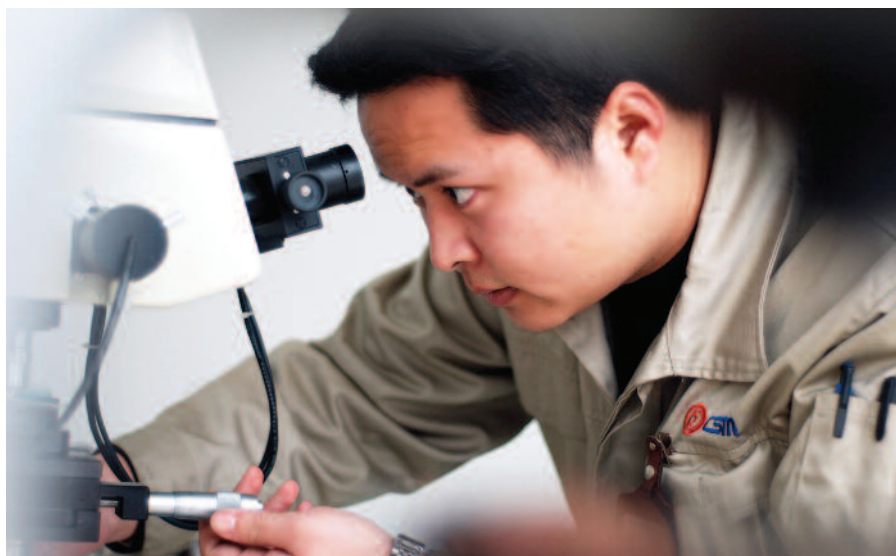
Testing the microstructure of the metal on the production premises.
