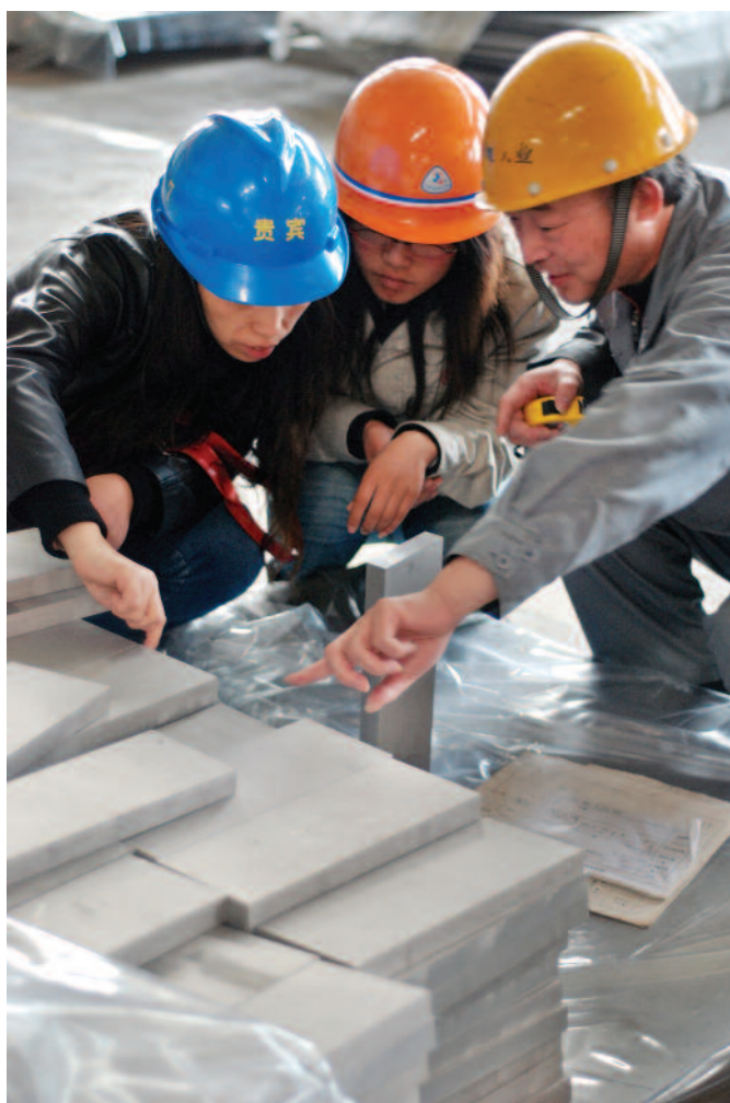
Checking the surface quality of the titanium target plate.
