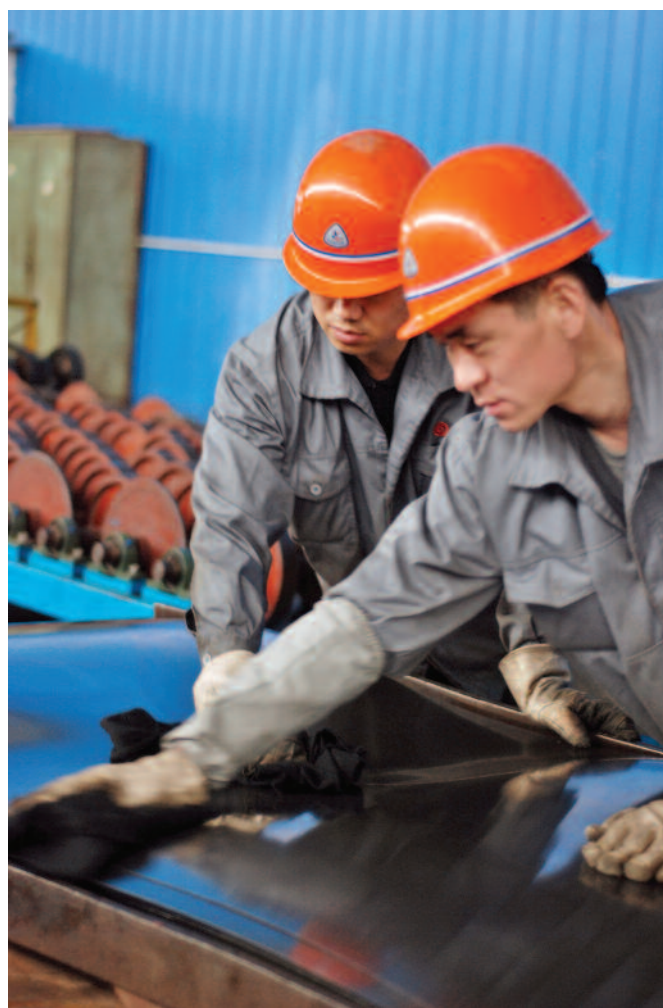
Cleaning before annealing.
