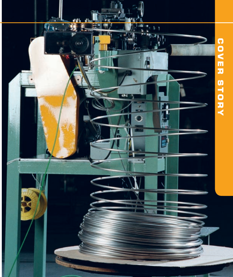
Alloy 825 down-hole control line tubing being manufactured at the North Branch, New Jersey facility.
