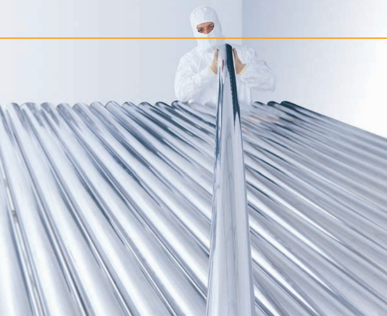
RathGibson High Purity tubing undergoing "cleanroom" inspection at the Janesville, Wisconsin facility.
