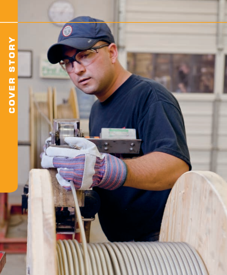
Down-hole 316L control line tubing being reeled at the Mid-South Control Line facility in Marrero, Louisiana.
