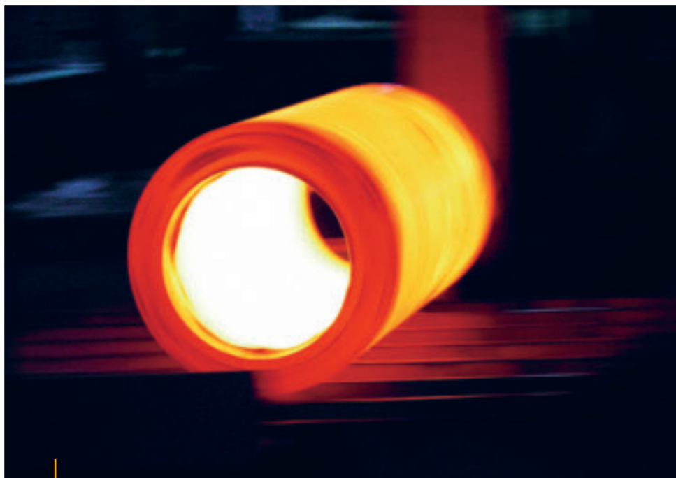
Billet ready for extruding.
