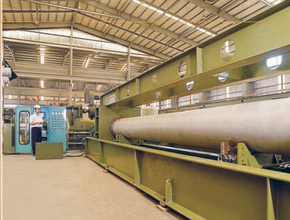
Froch can carry out a number of tests in its own facility, including hydrostatic testing for pipe up to 36" in diameter.
