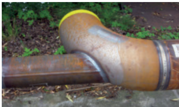
High quality prefabrication of metallurgically clad spools for a refinery.
