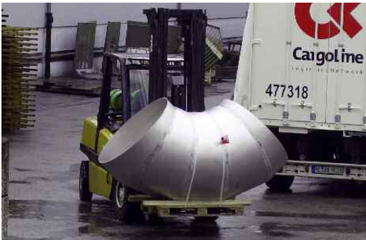
Fabricated elbow dia 1220 x 6,0 mm in Alloy 926
