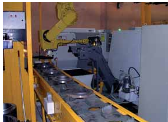
Forty-eight fully robotic CNC machining lines are being installed to increase the capacity for machined products by 300% to 300,000 pieces per month.
