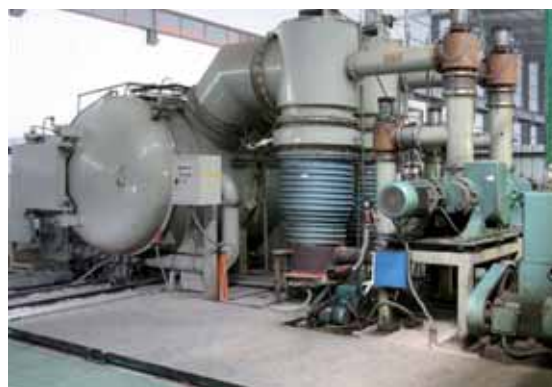
This is the essential equipment for PHE - Vacuum Annealing Furnace.
