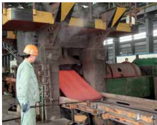
Hot rolling tubes for chemical and petroleum refinery plants.
