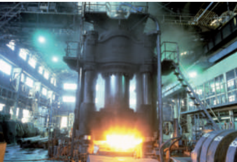
The vertical piecing press provides large diameter pipes (with an outside diameter of up to approximately 950 mm) that satisfy demands not only for nuclear and fossil power boiler applications, but also for chemical applications.
