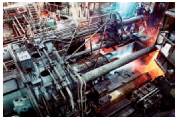
The hot extrusion mill is highly efficient for producing hot finished pipes.
