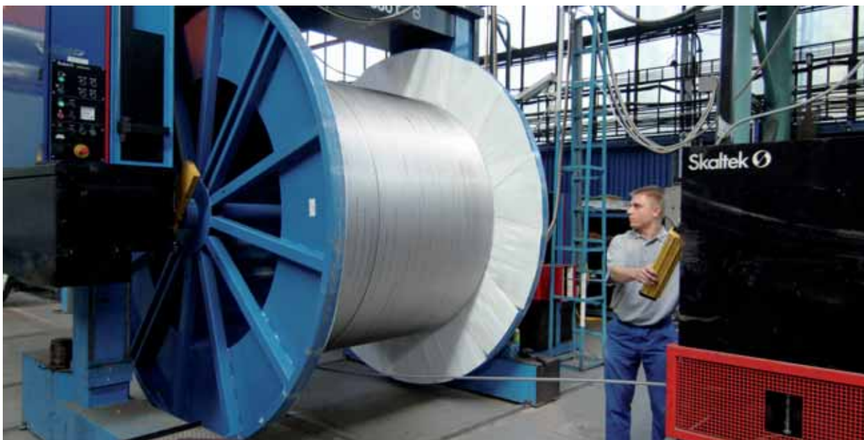
In the Czech Republic, Sandvik has a highly specialized unit for the manufacturing of seamless coiled tubing in lengths up to 15 kilometres. These tubes are used in umbilicals in the oil and gas industry - and the materials used have been developed to withstand extreme pressure and high temperatures at depths of more than 7,500 ft. without maintenance.
