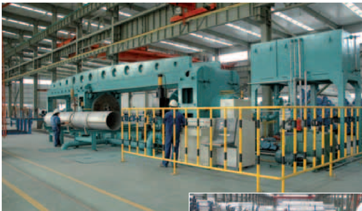
Hydrostatic testing facility
