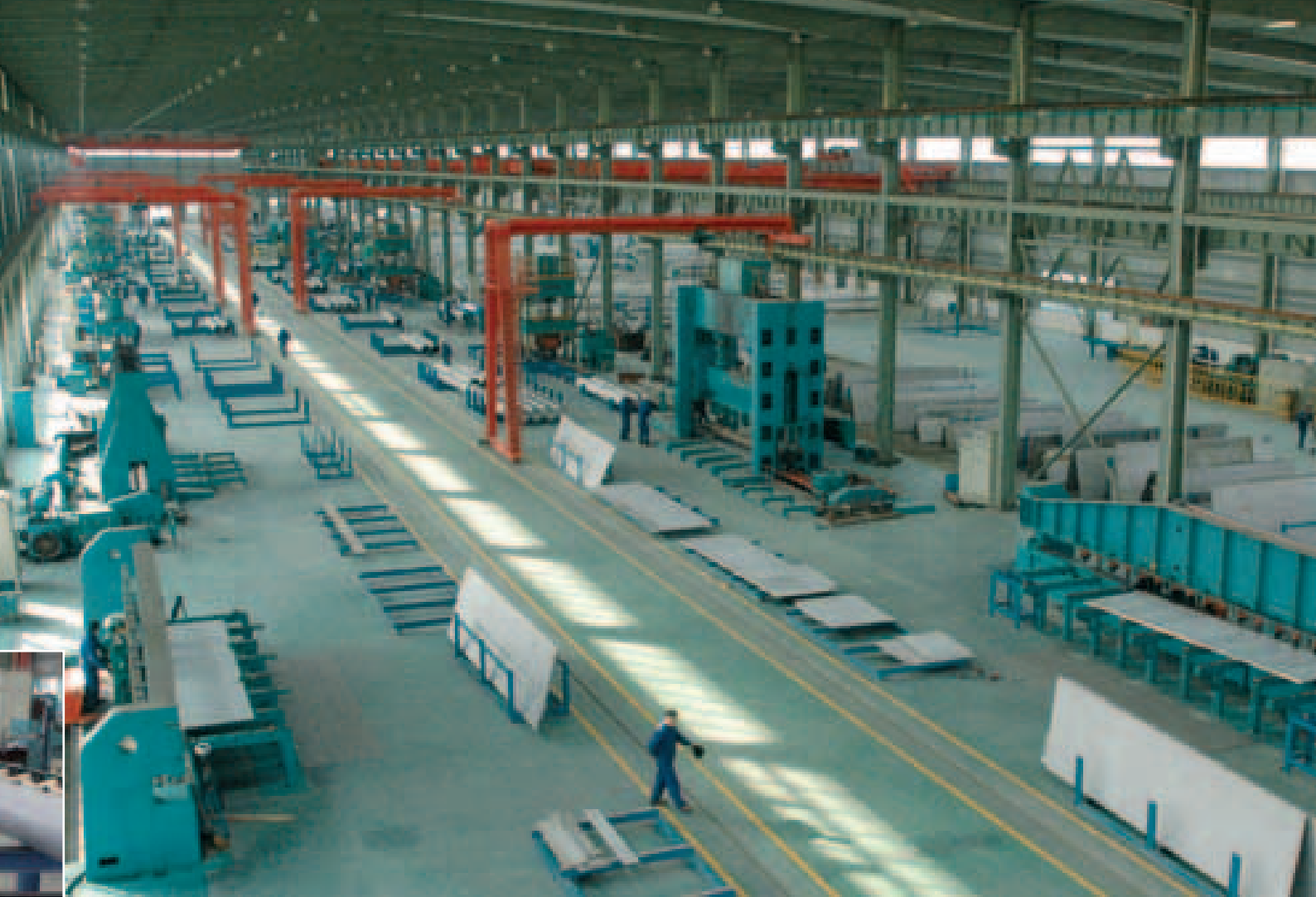
The workshop for large diameter welded pipes with state of the art pipe welding, X ray and hydrostatic testing equipment.
