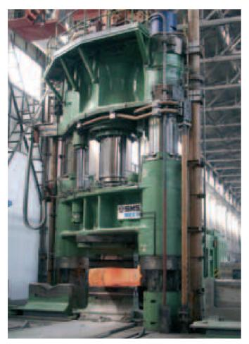
Significant investments can also been seen in the new forging workshop which houses both a Chinese-made forge and, also since May 2004, a German-made forge press. Equipment in the forging workshop now includes an SXP-13 precision forging press, a ring rolling mill, a 3150 ton hydraulic press and a 2500 ton high-speed hydraulic press that enables Baoti to produce titanium and titanium alloy bars, billets, discs and rings. tal research and development of titanium alloys and applications.
