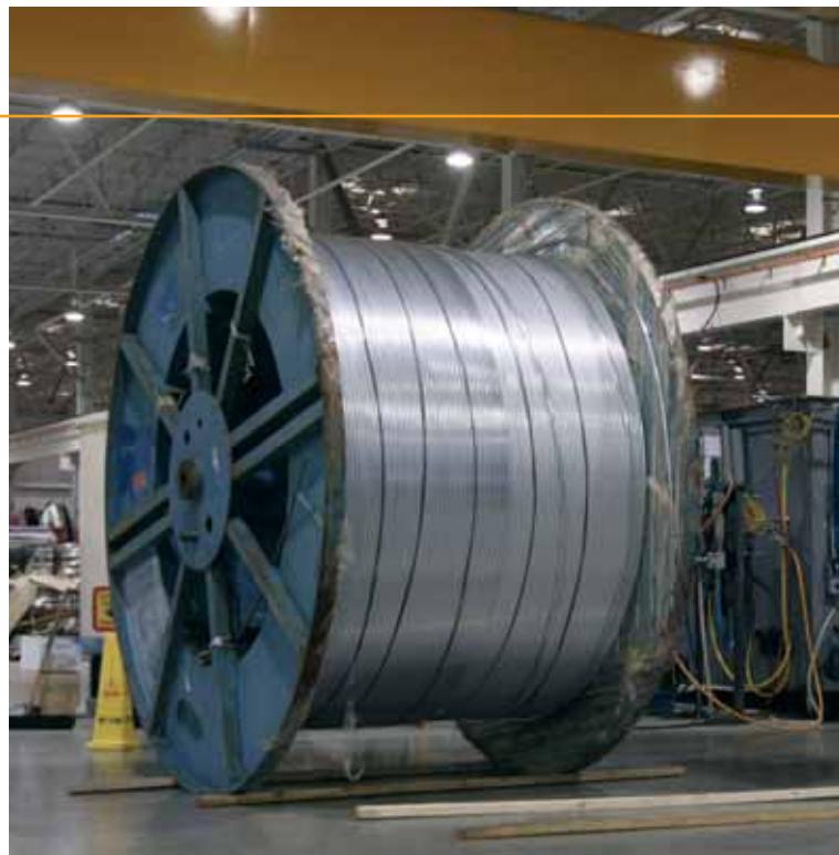
A reel containing 30,000 feet of RathGibson Zinc Clad, lean duplex subsea umbilical tubing which is being prepared for shipment. (June 2005)
