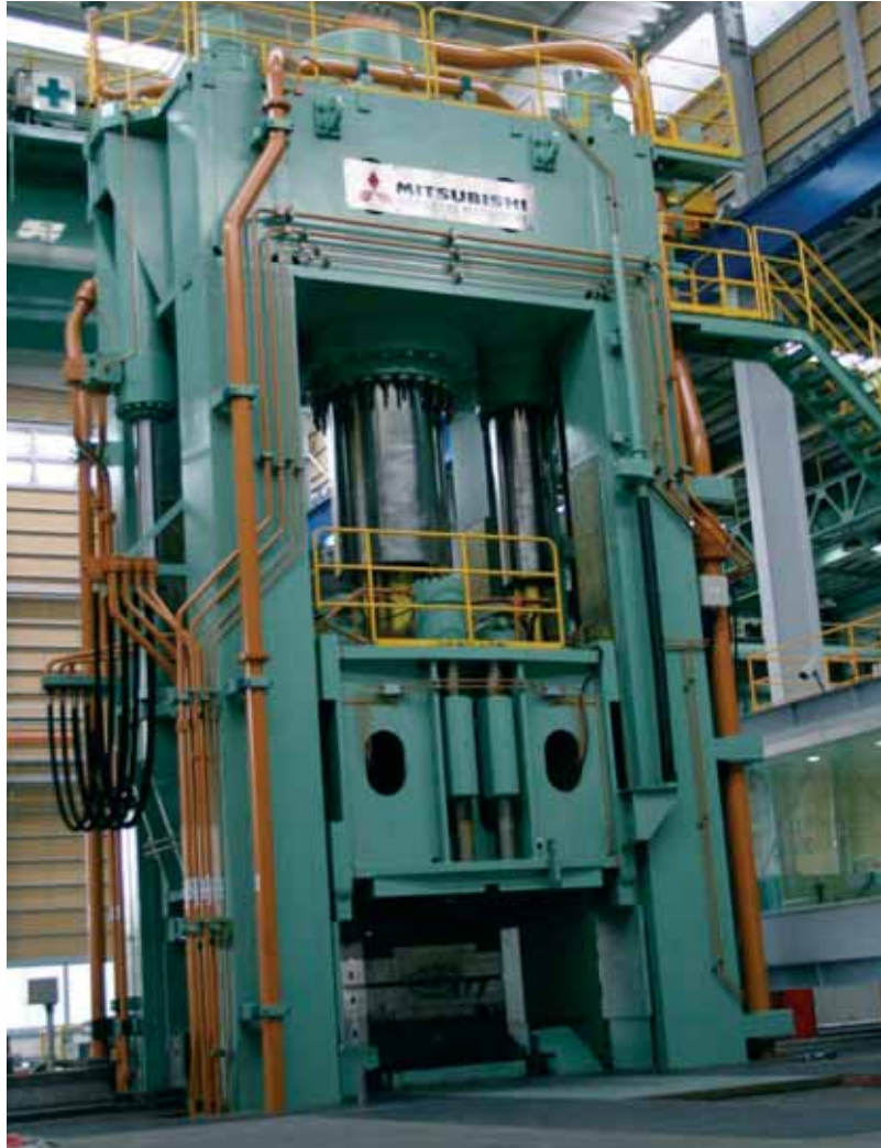
Mitsubishi Materials recently installed a 7000-ton high-speed forging press at the Okegawa plant.
