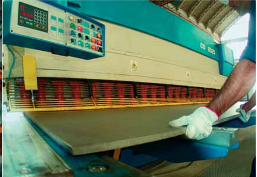
Torresin Titanio has water-jet cutters, guillotine shears with a cutting capacity of up to 6 metres, a flattening and coil cutting line, band saws for cutting tubes and saws for cutting bars up to 350 mm in diameter.
