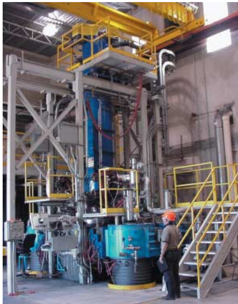
ATI Wah Chang's new niobium furnace located in Albany, Oregon. First year in production 2003. It enables growth in niobium products, such as Medical - MRI and High-energy physics.
