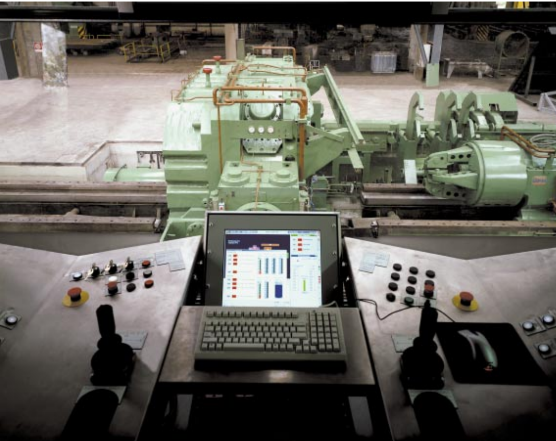
Italfond's brand new peeling machine will be operational in May 2004. With the new forging and peeling machines Italfond can improve lead times for bars up to 330mm significantly.
