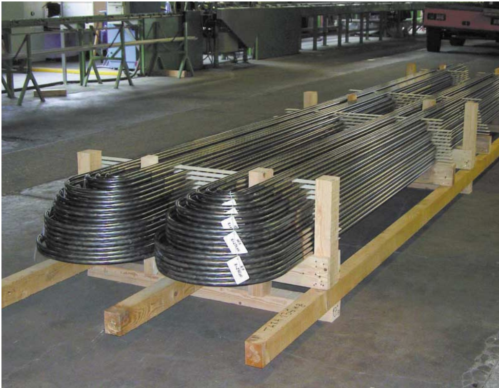
TPS stocks more than 300.000 metres of heat exchanger tubes in carbon, low-alloy, stainless steel, brass and copper nickel.
