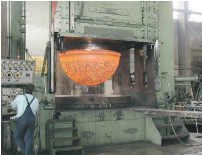
Hot pressing of a hemispherical head Øi 1600 x165 mm.
