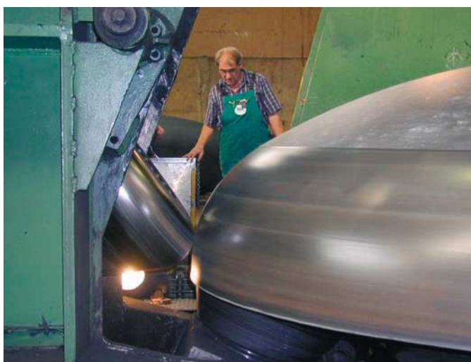
Spinning of elliptical head 2:1 Øi 3.600 x 12 mm. Material: Titanium Gr. 2
