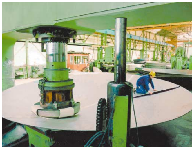
Dishing of stainless steel head.
