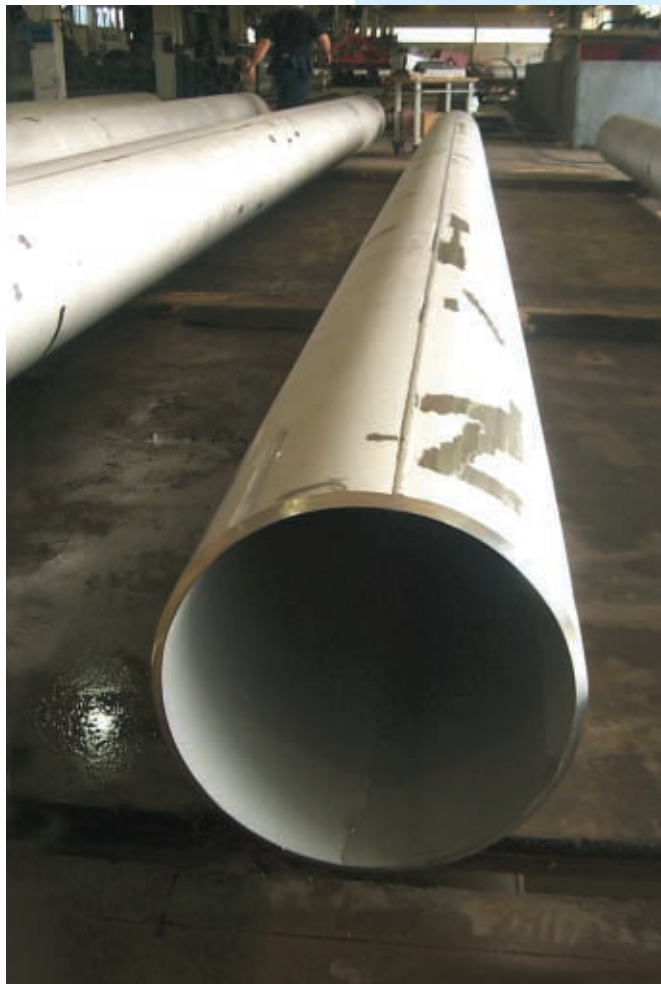
This year Inox Tech completed a unique project for the manufacturing of 12-metre long pipes with only one welding seam.
