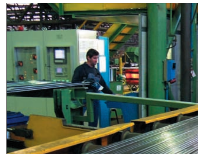
Operating at up to 1230°C, the new open air furnace offers productivity and quality improvements as well as widening the range of materials that can be offered. It can also easily accommodate tubes of up to thirty metres, the maximum length that can be produced at Costa Volpino.
