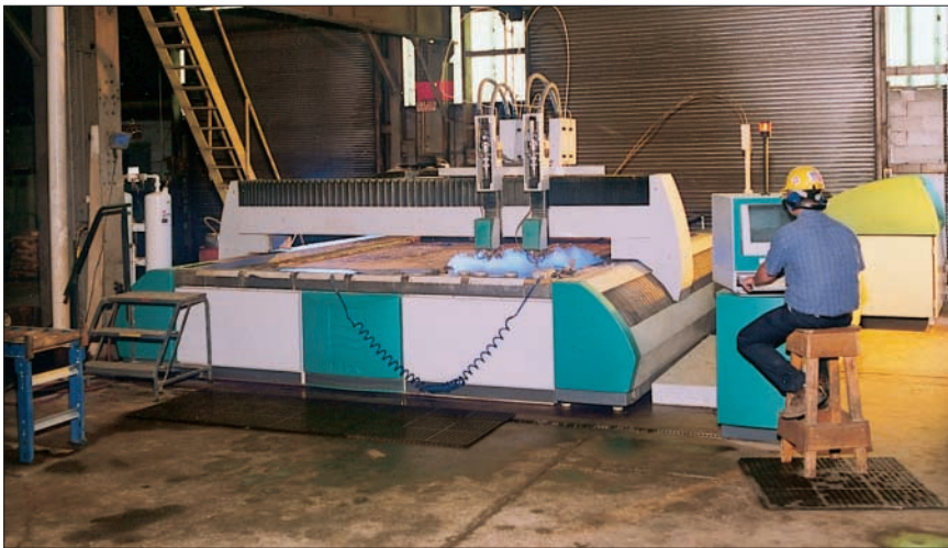
A new state-of-the-art waterjet cutting system enables the Steel Division to supply cost effective, near net shape parts from specialty plate.
