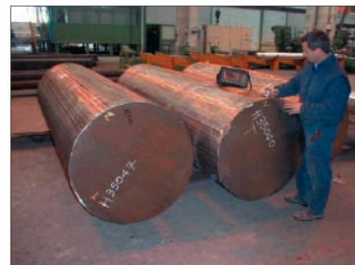
**Italfond can produce a wide range of stainless steel grades, mainly martensitic, austenitic, superaustenitic, duplex and superduplex, and nickel-based alloys. In terms of shape and size, the company produces round and square bars, from small to very large diameter (5 to 32 inches).**
