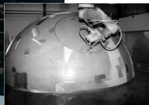
Hemisphere in nickel alloy cut by water by Bibus' subcontractor Waterjet.
