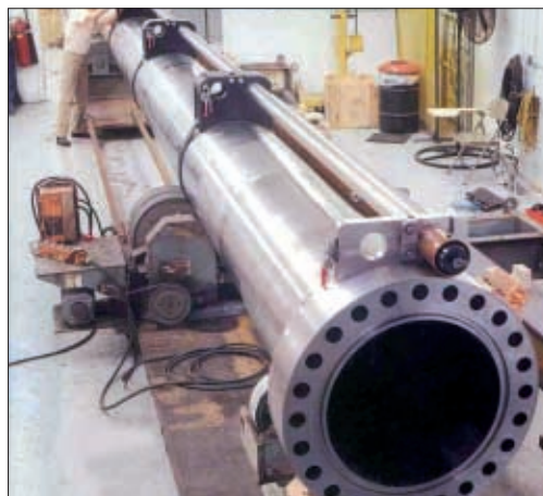
A drilling riser in production at RTI Energy Systems.
