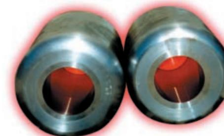
**X65/825 Extrusion Billets for KLAD seamless pipe.**
