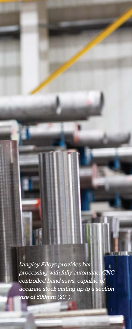
Additional in-house services include deep hole boring, machining and CNC-controlled bands saws, capable of accurate stock cutting up to a section size of 500mm (20").
