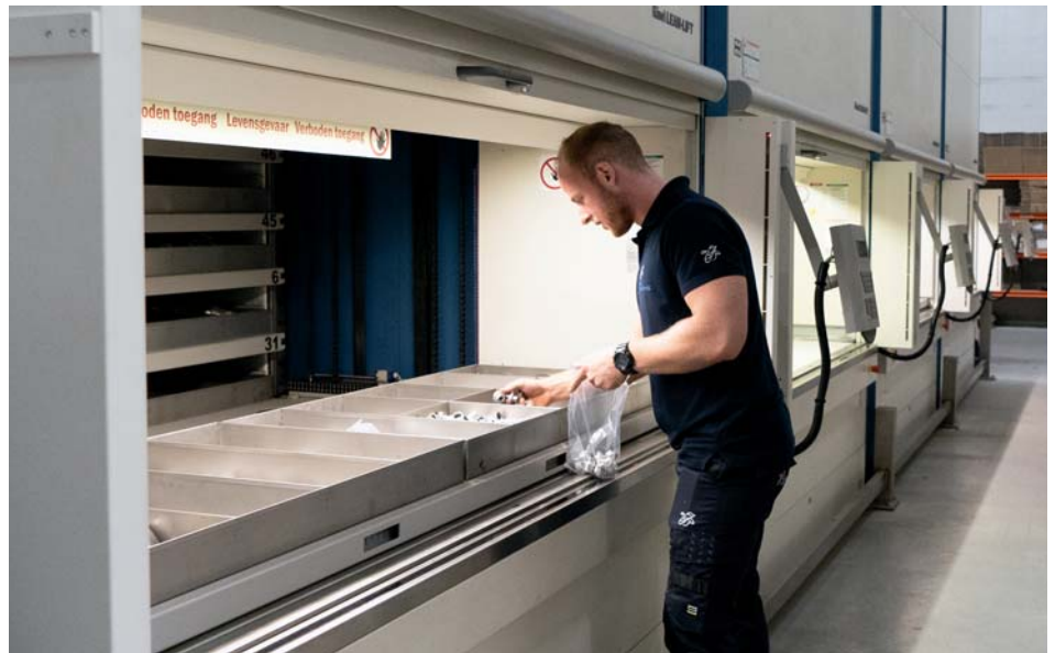
The high-tech order picking department is dominated by several huge lifts which automatically pick up trays of products and present them at exactly the right height for the machine operator to access.
