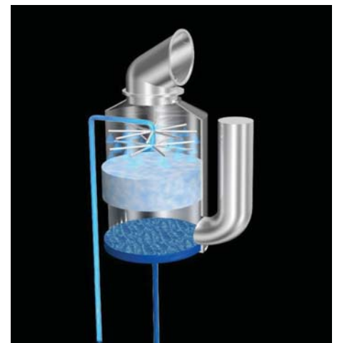
SOx scrubber for ship.
