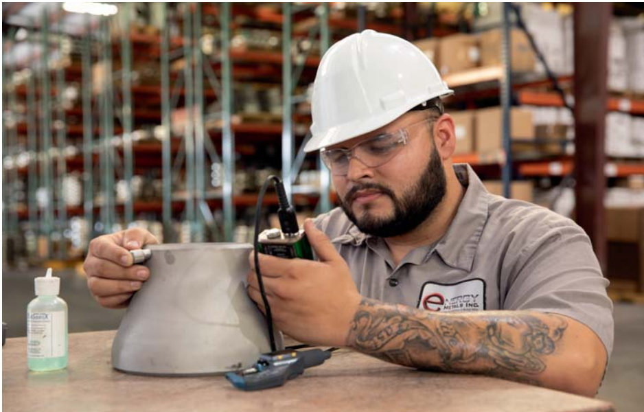
A key component of the Quality Program is in-house Positive Material Identification (PMI) and digital wall measuring equipment
